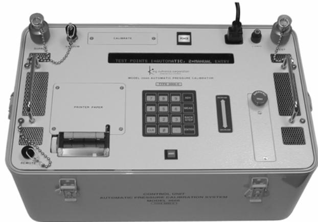
An easily readable vacuum-fluorescent front panel display provides information such as the target pressure, actual pressure, and pass/fail status for the unit under test. Hard copies of test and calibration results can be quickly generated using the built-in printer.
