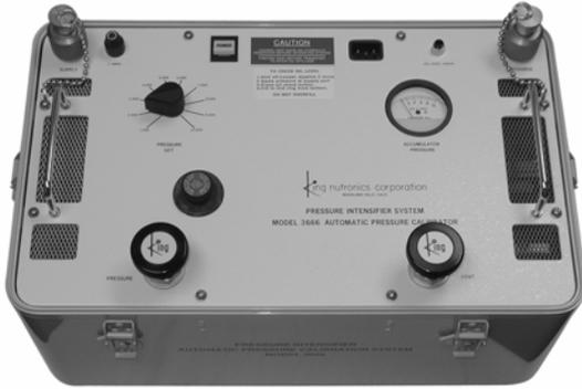
The Model 3666-17-1 Pressure Intensifier is an electrically powered device that accepts low pressure gaseous nitrogen from 500 to 2,216 psi and boosts the pressure up to 10,000 psig in 1,000 psig increments for use by the Model 3666 APC control unit.
